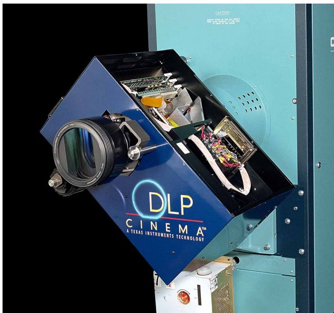
Figure 1.19 Digital Light Processing™ cinema projector attached to a standard lamp housing Image courtesy Texas Instruments, Inc.
