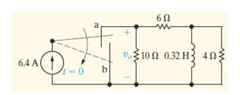
$$i_0 := 6.4 \text{A} \cdot \frac{(10 \parallel 6)}{6} = 4 \text{ A} \qquad i_L(t) := i_0 \cdot e^{\frac{-t}{\tau}} \qquad v_0(t) := -i_L(t) \cdot R \cdot \frac{10\Omega}{16\Omega}$$
