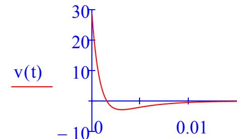
b) Given  $t_{zv} := 1\text{ms}$        $v(t_{zv}) = 0$        $t_{zv} := \text{Find}(t_{zv}) = 1.54\cdot\text{ms}$
