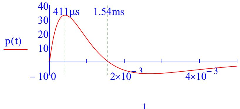
$$d) \quad \text{Given } t_{pm} := 0s \quad \frac{d}{dt}_{pm} p(t_{pm}) = 0 \quad t_{pmax} := \text{Find}(t_{pm}) = 411.051 \cdot \mu s$$
