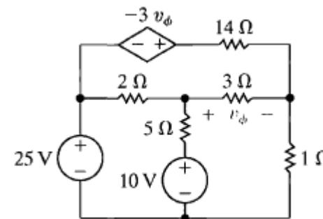
AP 4.9 Use the mesh-current method to find  $v_o$  in the circuit shown.
