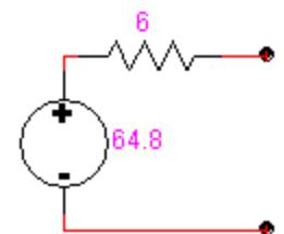
AP 4.17 Find the Norton equivalent circuit with respect to the terminals a,b for the circuit shown.
