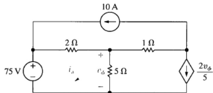
AP 4.12 Use the mesh-current method to find the power dissipated in the  $1 \Omega$  resistor in the circuit shown.
