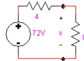
AP 4.16 Find the Thevenin equivalent circuit with respect to the terminals a,b for the circuit shown.
