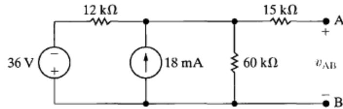
AP 4.19 Find the Thevenin equivalent circuit with respect to the terminals a,b for the circuit shown.
