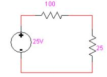
b)  $R_L := 25\Omega$   $V_L := \frac{25}{100 + 25} \cdot V_{th} = 5V$   $P_{tr} := \frac{V_L^2}{R_T} = 1W$
