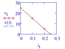
$I_{sc} := 0.25A$   $R_{sc} := \frac{V_{th}}{I_{sc}} = 100 \Omega$ a)  $V_{th} := 25V$
