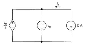
b)  $P := -i_b \cdot v_g = -16 W$  power is delivered by the current source
